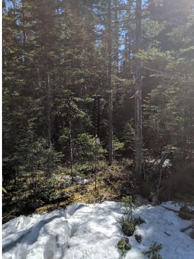
Lindgren Funnel trap, equipped with Hobo® Temp/Light Pendant to monitor the effects of light intensity on beetle flight. Uschenko 2020.
