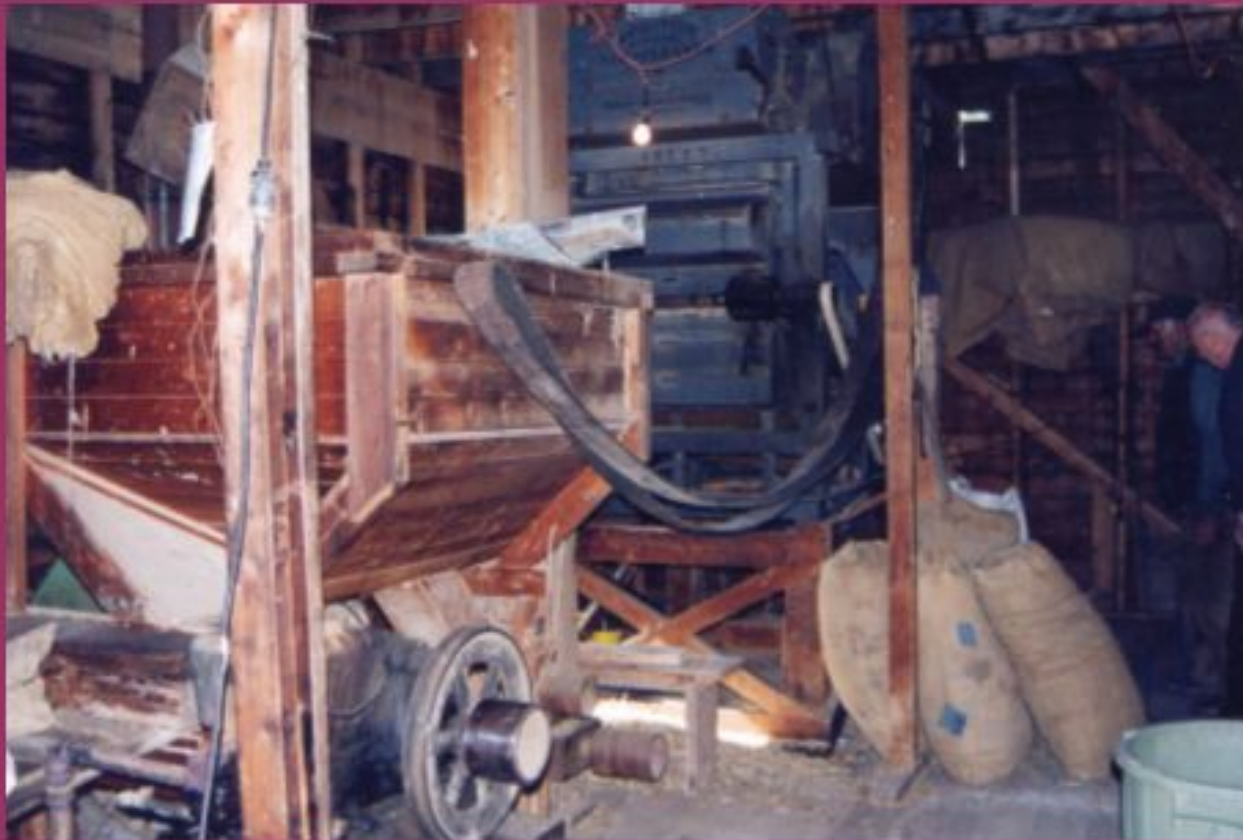
The hopper that the grain feeds into (1927 seed cleaning plant)
